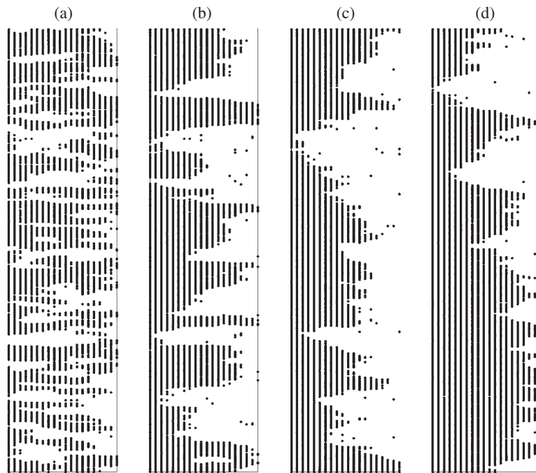
Figure 4. Typical snapshot configurations obtained during the dynamic evolution of the film towards the stationary state. The lattice size is L = 20 , D = 512 and the snapshots were obtained for h_w = 0.7229 and T_w = 0.700 . (a) t = 10 mcs, (b) t = 80 mcs, (c) t = 300 mcs and (d) t = 20\,000 mcs. Note that the scale of the coordinate along the films is chosen as a factor of 6.4 smaller than the scale perpendicular to the film.
